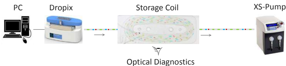
Schematic of setup required for making droplets in sequence. Arrows indicate direction of flow – the syringe pump works in withdrawal mode.
