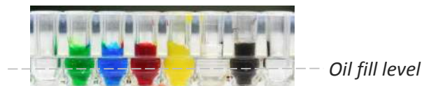
Sample holder and sample strip with 6 (out of 24) wells in use. Aqueous reagents loaded in 6 wells – Well#12 (green), Well #13 (blue), Well #14 (red), Well #15 (yellow), Well #16 (clear), and Well #17(brown). Buoyancy and surface tension help retain the sample in the well.
