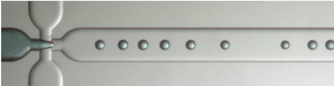
Image of water-in-oil droplets formed with a market leading syringe pump and Mitos Droplet Junction Chip - Hydrophobic
