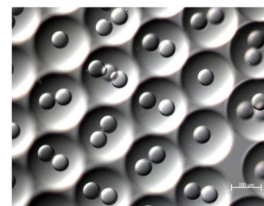
Adjustment of the three flow rates was performed to observe the range of droplet sizes that could be created. Although further work is continuing in this area, and not all combinations of inner and outer droplet diameter can be achieved with a single chip pair, it is possible to achieve inner droplet diameters in the range 25 to 50  $\mu\text{m}$  and outer droplet diameters of 150 to 200  $\mu\text{m}$ .
