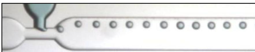
The X-Junction will produce droplets in the centre of the channel whereas the T-Junction has a tendency to push them towards the top. The T-Junction is often used to split a flow from a pump, and then the split flow is fed into two of the X-Junction inputs.
