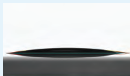
Water drop (8µl) on untreated glass slide, average contact angle of 7 degrees
