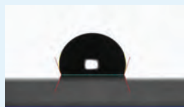
Water drop (8µl) on Pico-Glide™ treated glass slide, average contact angle of 107 degrees
