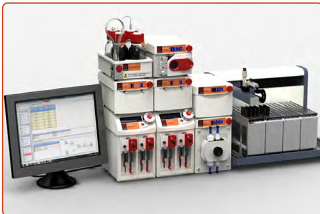
Left: Design and fabrication of a modular flow system for Syrris Ltd
